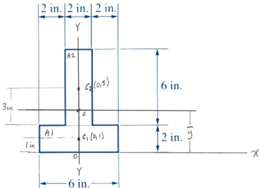
Define Reference Axis. The area is symmetric about the Y-Y axis, therefore the centroid must lie on the y-axis
